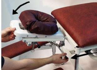
2-3. The adjustable arm rests are to be mounted on the chromed pipes. **NOTE! Don't screw on the locking handle when the fastener is not mounted on the pipe. The metal on the expansion function might be damaged.** The armrests are regulated both in height and side with a handle and an expansion locking for soft and efficient locking.
